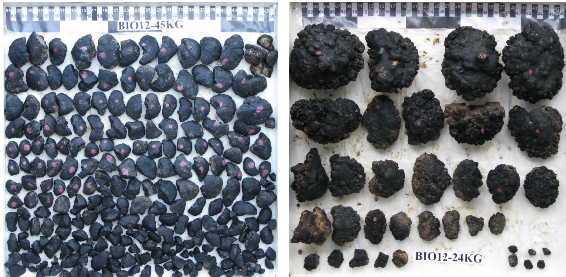
Figure 4.5: Box corer samples from an area dominated by small-sized nodules (left panel) and from an area dominated by large-sized nodules (right panel). These samples derive from a seafloor area covering 50x50 cm each. The differences in size, texture and number are clearly visible.
